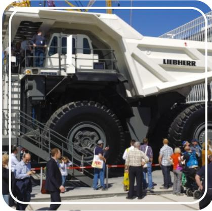
The Liebherr T 282C is the ultimate monster in automotive at the moment! It is the size of a house and its engine gives 3650hp. It weighs 252tons and can carry up to 400tons.
